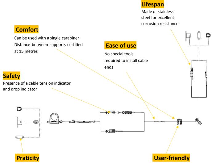
The starting post of the line can also be used as the finishing post, regardless of the number of corners and intermediate pieces (in the case of an ALTIFIX or PST support).
